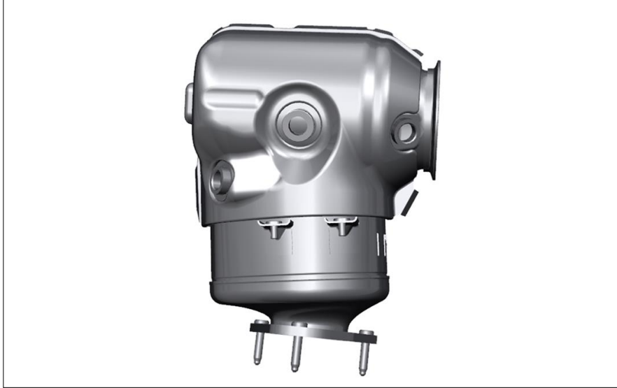
Fig. 3. A common Volvo PHEV Exhaust System, in this paper named Generation 2 (G2)
