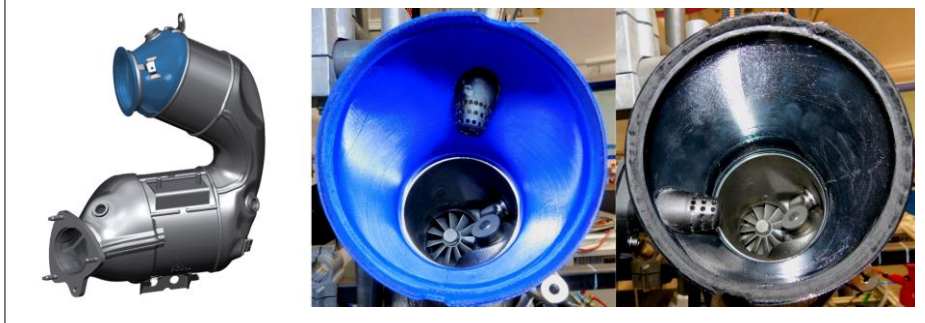
Fig. 17. 3D-printed Nozzle and G3 Inlet Cone, connected to the turbo charger, baseline 0° (left) and 120° (right) Nozzle Position
