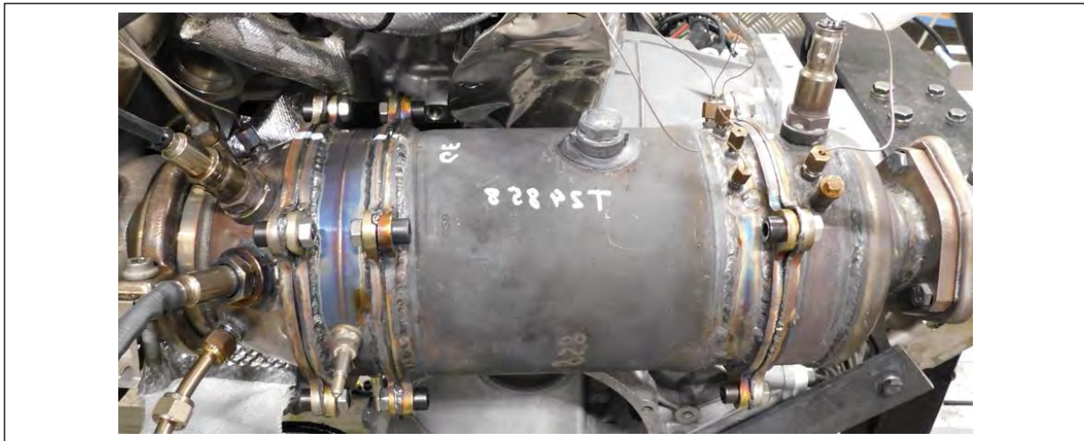
Fig. 20 The close coupled exhaust aftertreatment with (from left to right) the mounted EHD and the original catalytic converter. It is possible to see also the flanges for the EHD mounting.
